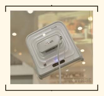
the robots drag cleaning fluid and wipers along the surface in regular patterns. They work their way up and down cleaning the whole windows at a time. This method is not only safer but also more efficient because the robots don't need to stop for lunch or to adjust the height of staging.
