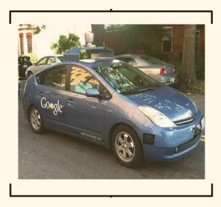
all without an accident. To perform its driverless functions, the control system of the car calls upon many sensors with capabilities ranging from **ultrasonic** to imaging. Even though this car has proven to be safe on the roads, it will have to demonstrate many more road tests in order for it to be legalized around the nation and be brought into the consumer market.
