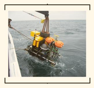
The researchers tell the robot where to go, and the robot uses propellers and jets of water to move around. If something interesting float past, the robot has containers and suction tubes to collect it. With their small design and long battery life, the robots allow scientists to explore shipwrecks and sea vents for hours.
