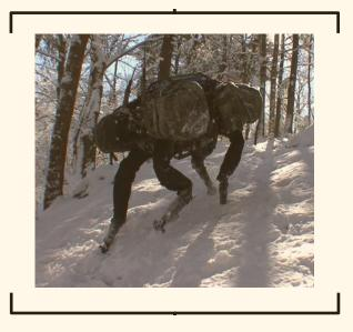
Big Dog uses a **gyroscope** as well as a group load sensor and shockabsorbing legs to keep balance. In addition, this military grade robot has an arm which can manipulate very large loads which has the intended use to transport wounded soldiers during battle. The strength of this appendage has been tested by throwing cinder blocks many yards.
